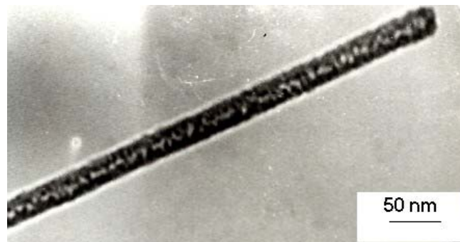
Figure 3: Transmission electron micrograph for specimen1 showing single multi-walled carbon nanotube.
